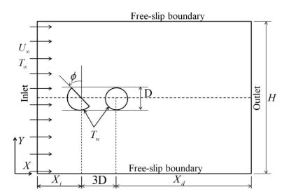
The angle of incidence of the semi-circular cylinder is  $\phi=45^\circ$ . The upstream, downstream distances and the height of the domain are chosen to be  $X_i=8D, X_d=37D$  and H=20D. Here, D is the projected diameter of the semi-circular cylinder and the diameter of the tandem circular cylinder.
