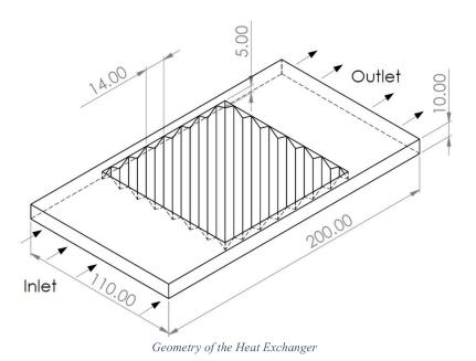
There are 14 equal sized corrugations present with the distance between the plates at the conduit entrance is 10 mm. Flowing fluid (water) is entering from inlet with velocity  $(0.07 \ m/s - 0.1 \ m/s)$  corresponding to the Reynolds number and exiting from outlet.
