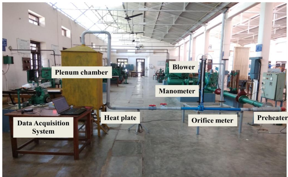
Fig. 1 Jet impingement test facility
