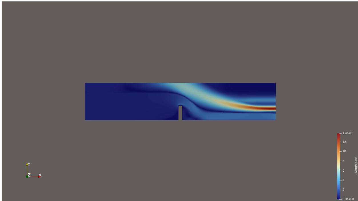
Figure 5: Velocity magnitude in the weir-only case showing the high-speed jet over the weir crest
