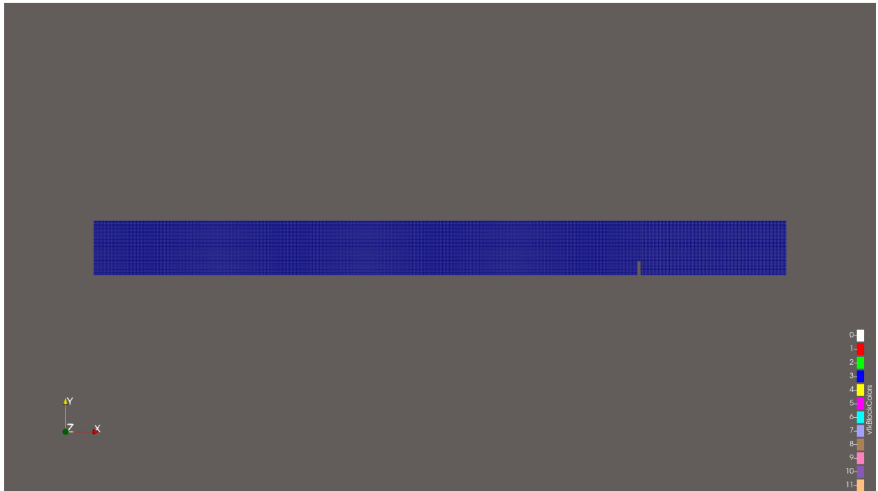
Figure 2: blockMesh grid showing the six-block structure
