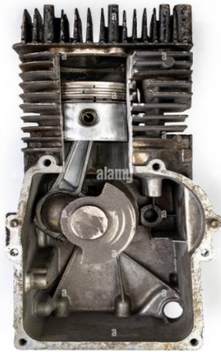
Fig 1: Cross-sectional view of an IC engine
