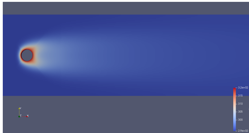
Figure 5: temperature contour of model at Re.no 20
