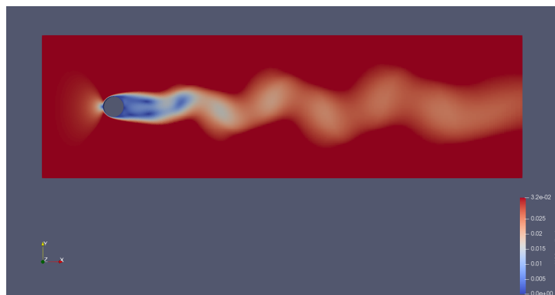
Figure 8: velocity contour of model at Re.no 200
