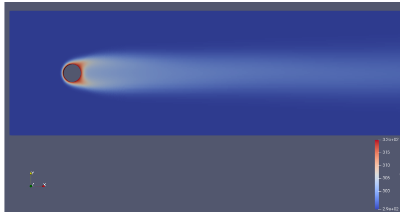
Figure 7: temperature contour of model at Re.no 100
