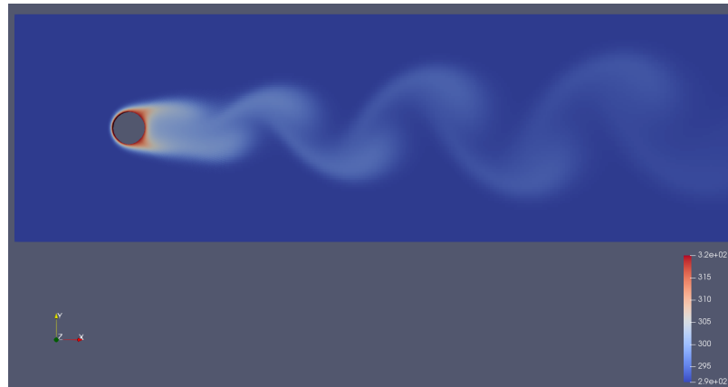
Figure 9: temperature contour of model at Re.no 200
