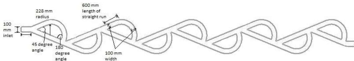
Figure 1: Tesla Valve with  $n$  diodic separation branches. There is no geometric difference in dimensions between the diodic separations. The only difference is in orientation and position.
