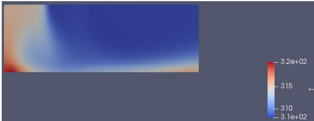
Figure 13 - Temperature profile of cross-section at the end of 90s
