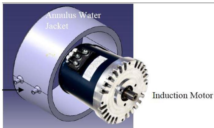
Fig 1 AC-50 INDUCTION MOTOR [1]
