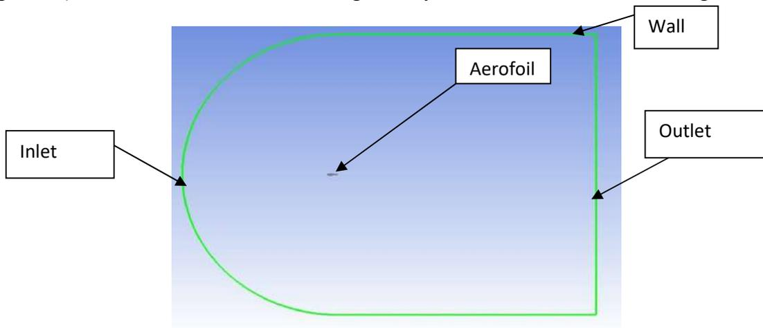
Figure 1. The geometry and Flow domain
