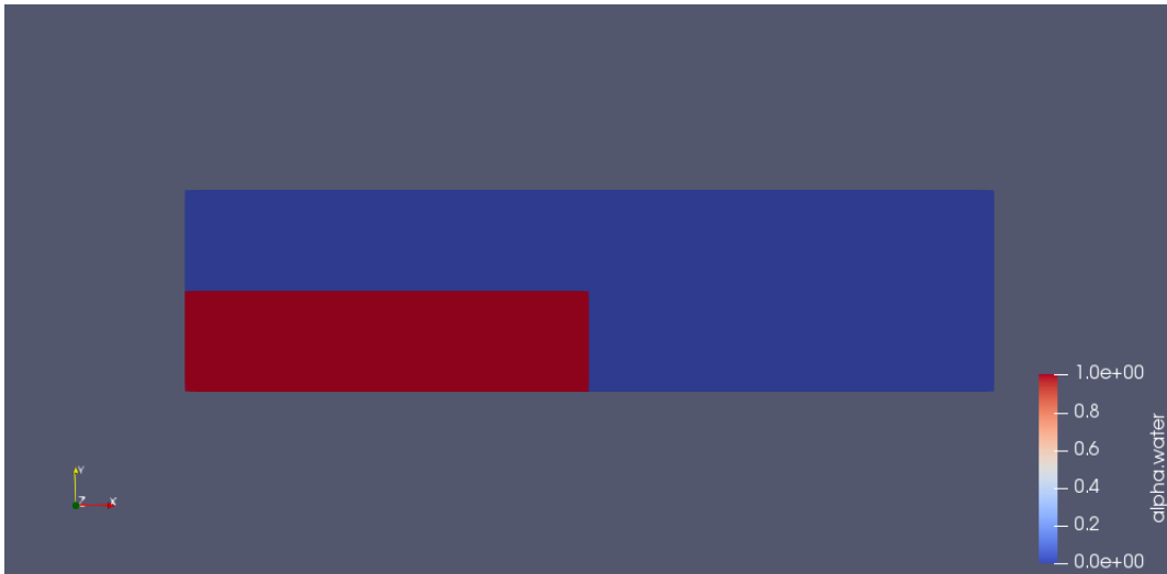
Figure 4: The two fluids at initial time for partial depth lock release
