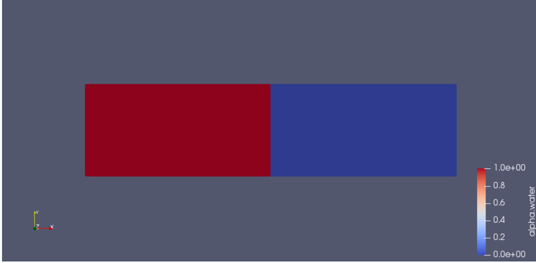
Figure 3: The two fluids at initial time for full depth lock release
