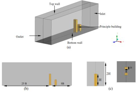
Fig.1: Geometry of the model and domain
