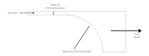
Figure 1: Geometry of the plain wall jet
